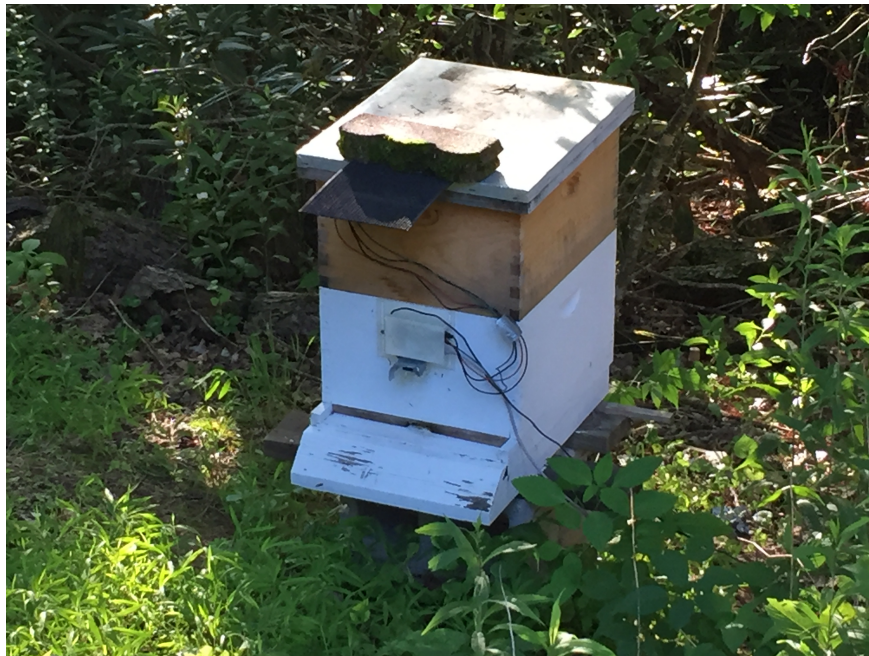
Figure 5.1: An example of a Raspberry Pi 3 data acquisition system
